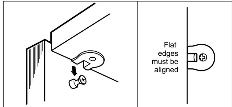
Flat edges must be aligned
