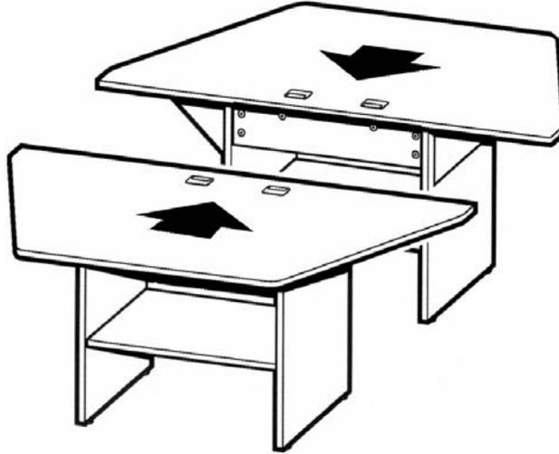
2. Align the tops together. Adjust the Levelers (H5) to level both Workstations at the same height.
