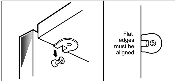
Using a #3 Phillips screwdriver, turn the rotating portion of the Rafix Cam a 1/2 turn clockwise to secure. **IMPORTANT!** Do not exceed 1/2 turn when tightening cams. Turn 1/2 turn counterclockwise to disassemble and remove panel.
