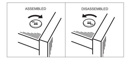
Insert 7 Minifix Cams (H1) into cam holes on Back (D) and 7 Minifix Cams into the Fixed Shelf (G) so that the arrows are facing out. Screw in 3 Minifix Bolts (H2) in the Back Panel as shown.
