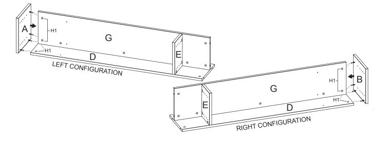
Insert Left Side (A) or Right Side (B) onto Back (D) as shown. Turn the connecting Minifix Cams on the Back clockwise to secure.
